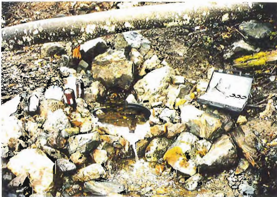
Photo #72: Closer 11/11/99 view of the APC/Sitka landfill's leachate sampling site #1 along its northwestern embankment toe. The sampling site consists of an 18"-dia. plastic pipe with a sampling depth of about 12" and an overflow notch to measure leachate flowrate.
