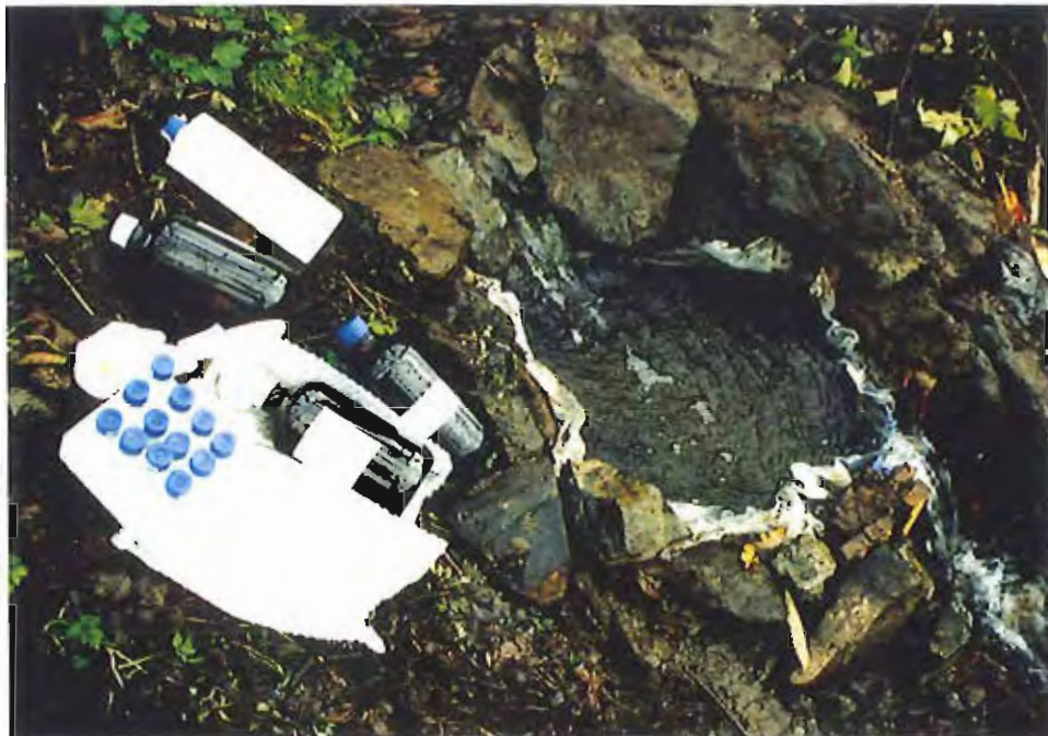
Photo #74: Closer 11/11/99 view looking down on the APC/Sitka landfill's leachate sampling site #2 located at about Sta. 5+20', showing its 18"-dia plastic pipe and its discharge notch.
